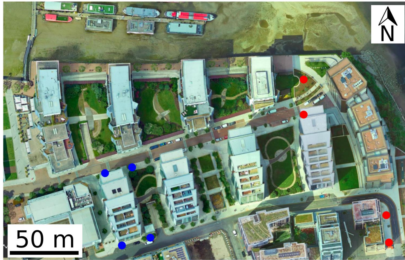
Figure 1: Plan-view of WRQ with cold wells shown in blue and warm wells shown in red.
