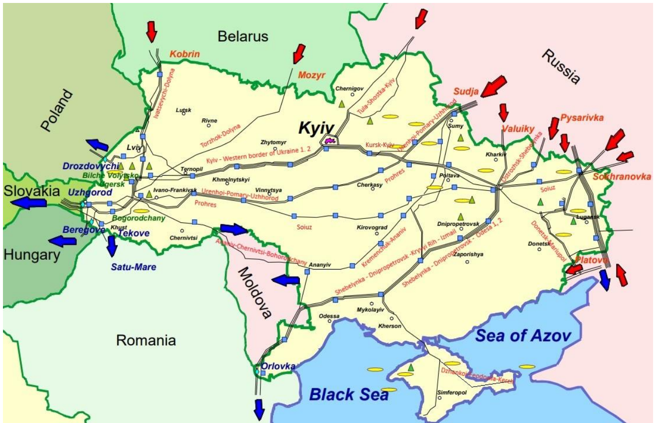
Fig. 4. Gas Transmission System of Ukraine [9].
