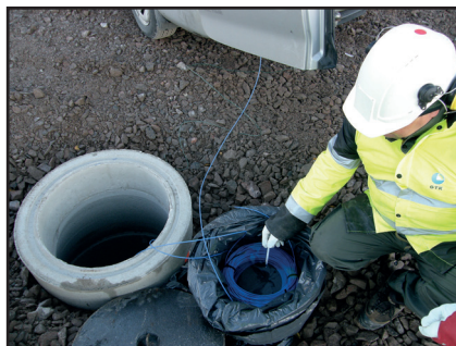
Fig.4 The boreholes in Sipoo are monitored online by optical fiber measurements (©GTK)
