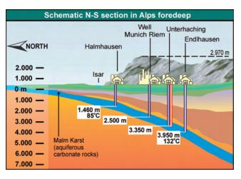
results were very favorable for the installation of a CHP plant of 3.5 MWe installed electrical capacity. The producing well drilled the hot aquifer at ~3 350 m; the water yield is 150 I/s with a temperature of 122°C and the water level lies at about 100 m below the surface. The reinjection well, drilled a few kilometers away, encountered even greater temperatures of water (at a depth of 3577 m).
